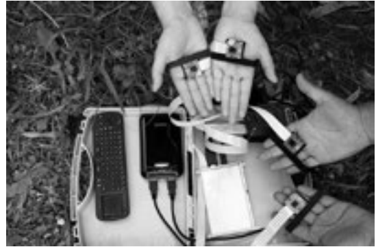
Figure 2. Haptic Cameras: basic operation hardware. Raspberry Pi running open source software, 4 cameras, battery, cables and LCD screen
