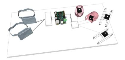
Figure 2. Prototype equipped with: a Raspberry Pi running on Linux, a portable battery, an LCD screen, VR goggles and 4 cameras custom-designed with 3D technology to "touch", or scan, and attached to users' hands; lenses are customized to take macro shots of surfaces. Device captures realtime footage of one or more users performing filming.]
